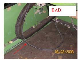
Numerous customers are sustaining <u>serious damage</u> to their machines OT switch arms due to miss routing of the table grease hoses. <u>Corrective Action:</u> Secure and route grease hose to the inside of Vacuum hose ensuring that upon full +/- stroke, hose remains away from OT dog arm.
