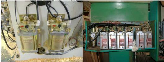
Greased Motors: Must use correct lubrication and DO NOT OVER GREASE. Mixing of greases, incorrect greases or over lubrication will cause premature failure of motors. A more thorough explanation of greasing procedures is provided with a PM inspection by TSG.
