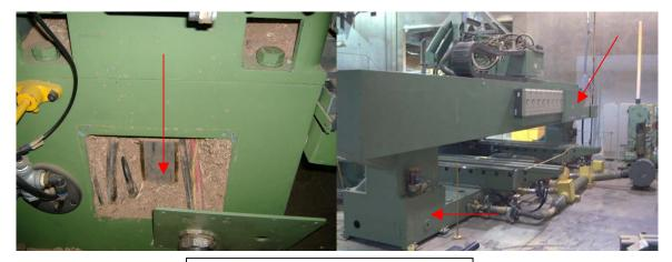
Electrical cabinets must be kept clean of debris and filters clean or changed on regular basis if applicable. Machines vary by model. Use vacuum cleaner. <u>Caution: Power must be removed</u> <u>from machine at main shut off.</u> <u>Use caution when using air due to</u> static discharge damage to circuit
